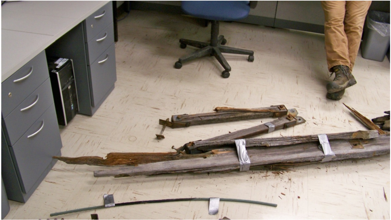
Photo B 4-25 Taken April 21, 2014. Removed failed double cross arm on Pole 24 of W185 on floor of Keene Area Work Center. Photo taken by NHPUC Safety Division
