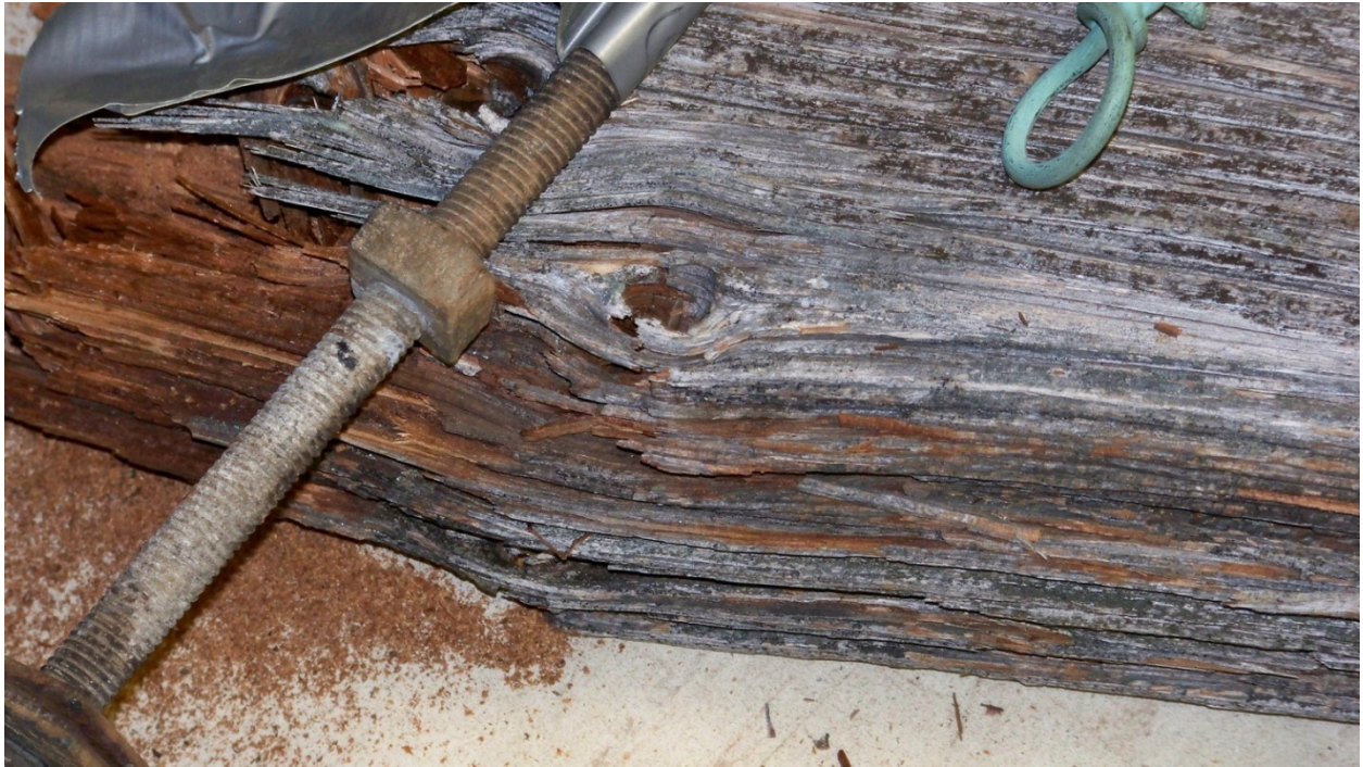
Photo B 4-23 Taken April 21, 2014. Remnants of failed double cross arm on Pole 24 of W185 on floor of Keene Area Work Center. Wood Rot is evident, bolts will no longer hold brackets on broken cross arm and supports Photo taken by NHPUC Safety Division
