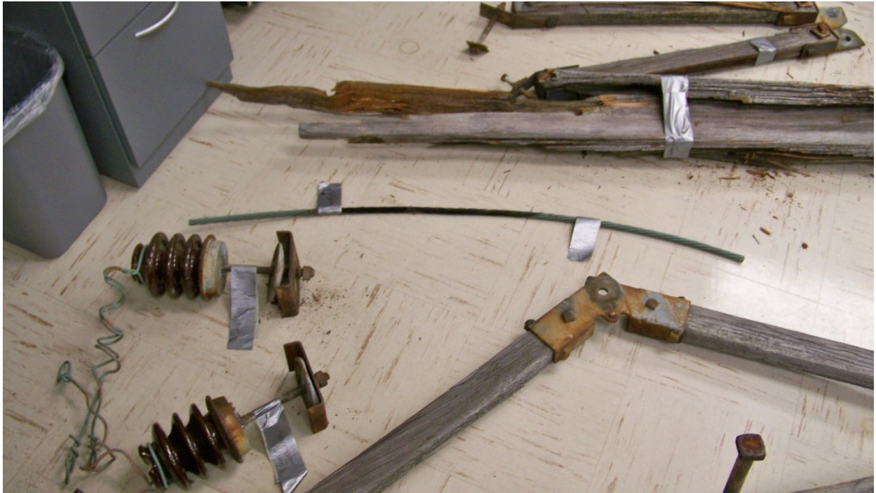
Photo B 4-22 Taken April 21, 2014. Components of failed double cross arm on Pole 24 of W185 on floor of Keene Area Work Center. Insulators, removed conductor (3 ft), broken cross arm and supports Photo taken by NHPUC Safety Division
