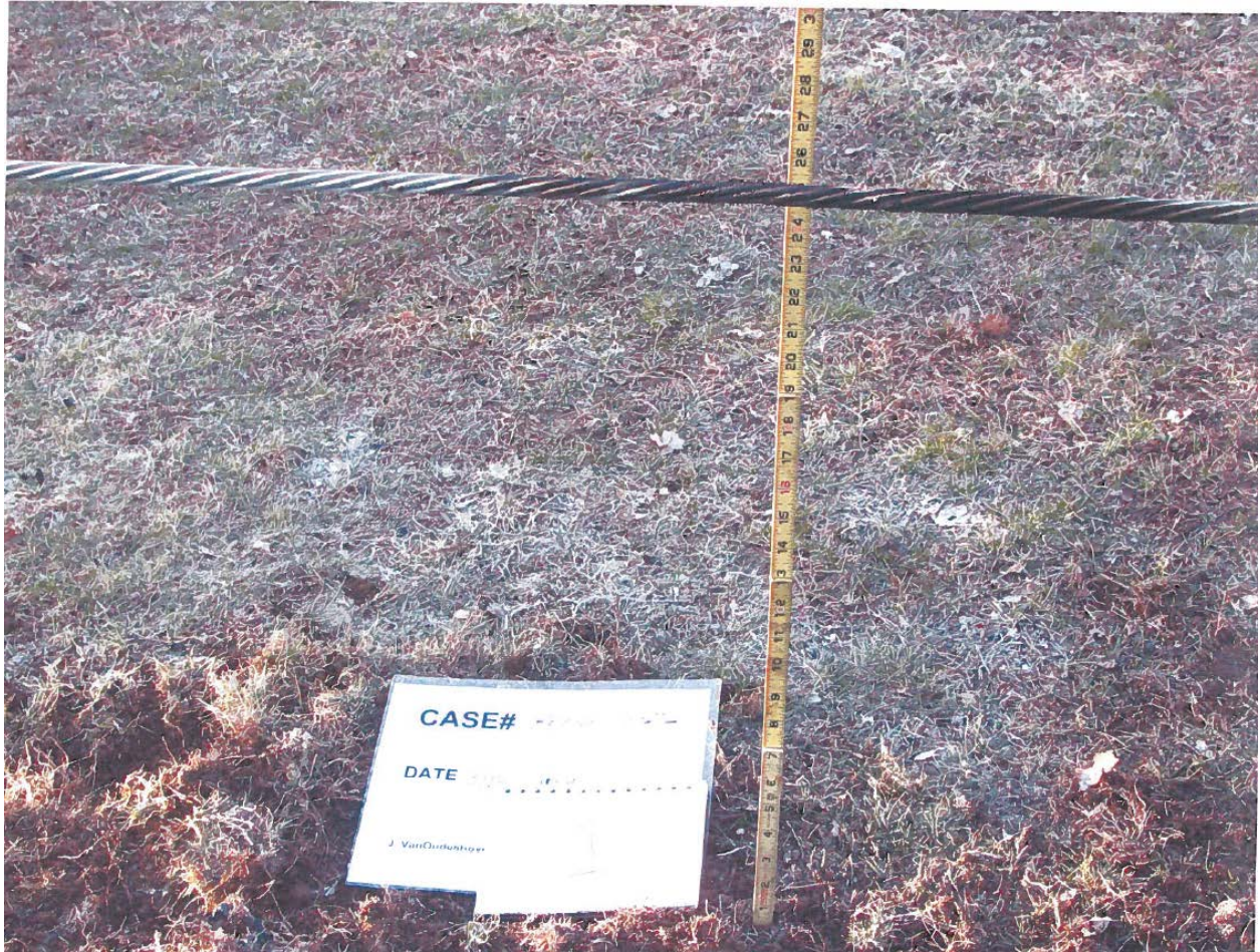
Photo B 3-14 Taken April 19, 2014 after contact was made. Closeup of the contact area. The primary conductor is of Phase 1 for W185 is approximately 24 inches above ground level. Photo provided by Public Service Co of New Hampshire
