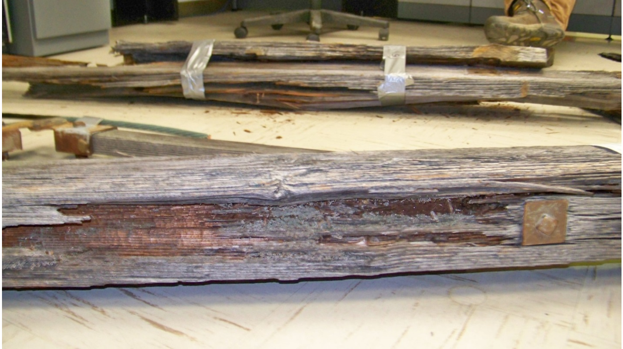
Photo B 4-24 Taken April 21, 2014. Remnants of failed double cross arm on Pole 24 of W185 on floor of Keene Area Work Center. Insect damage and wood rot witnessed on decayed broken cross arm and supports Photo taken by NHPUC Safety Division
