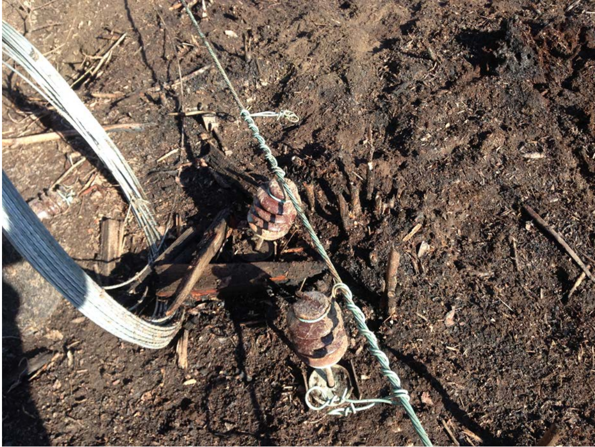
Photo B 2- 5 Close up of insulators from W185 phase 1 and portion of cross arm and conductor laying near bottom of pole 24. Insulators still attached to conductor but have completely pulled out from wooden cross arms. Spool of wire used for repair of guy wire is shown at left. Photo courtesy of NH State Fire Marshal's Office taken April 19 2014
