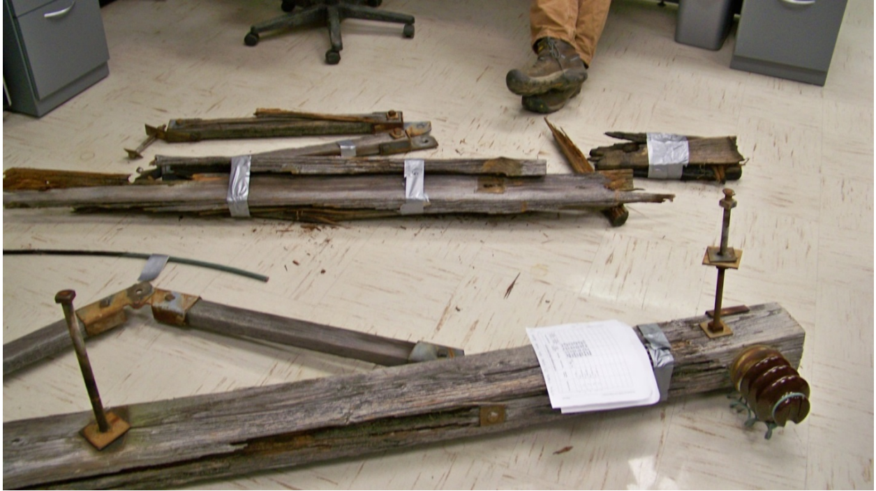
Photo B 4-27 Taken April 21, 2014. Removed failed double cross arm on Pole 24 of W185 on floor of Keene Area Work Center. Photo taken by NHPUC Safety Division
